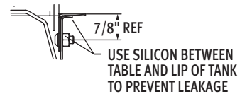
Sectional View Showing Table Connections
