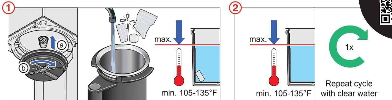
Attach the pacotizing® blade and spraguard, fill the pacotizing® beaker to the maximum fill line with 105-135 °F warm water, add a Pacojet Cleaning Tab, attach the pacotizing® beaker and protective beaker, start cleaning process.
