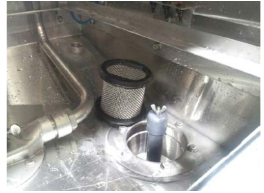
Placement of the pump filter into the drain sump
