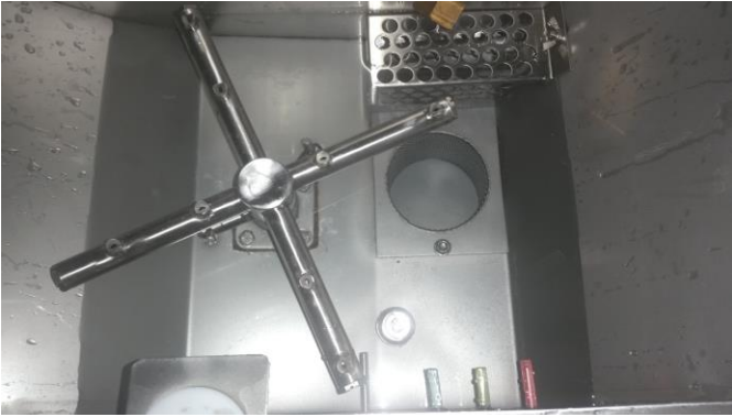
Wash tank with spray arm, float, secondary scrap screen
