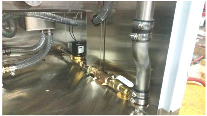
Showing 1/2" H2O solenoid, also stainless 1.5" drain tube
