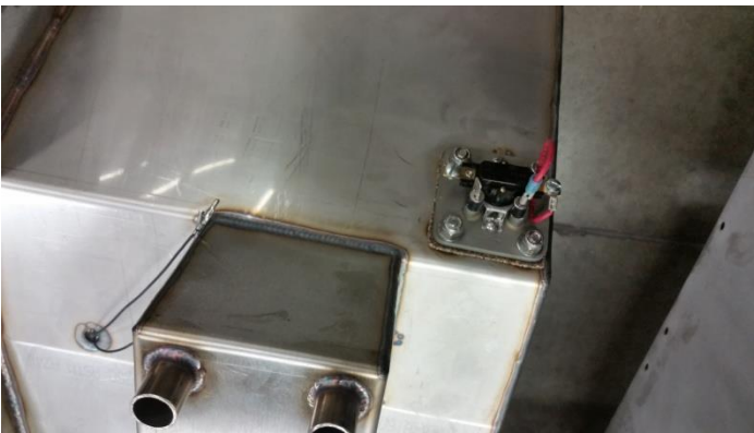
Showing bottom of tank, float wire, sump, heater attached
