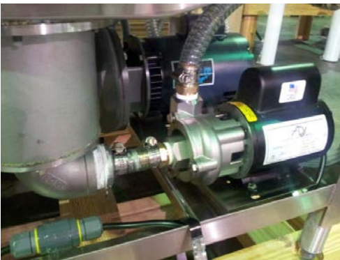
Showing stainless drain pump w/3/4" discharge tube
