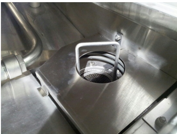
Sustainer heater cover and pump filter system
