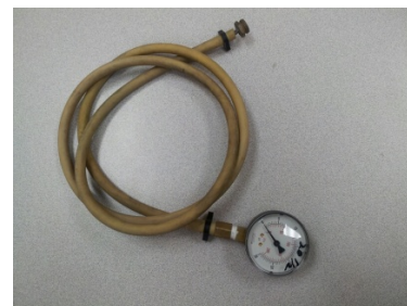
Spray arm pressure tester # 088-1048
