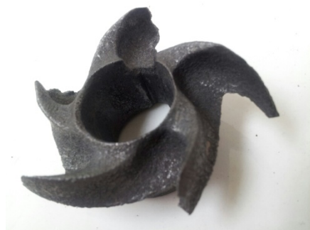
Impeller damaged from high acid solution
