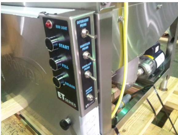
Showing controls on lower access door & drain pump
