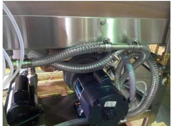
Drain "y" from overflow & drain pump, 60" drain tube
