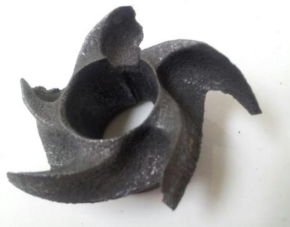
Impeller damaged from high acid solution
