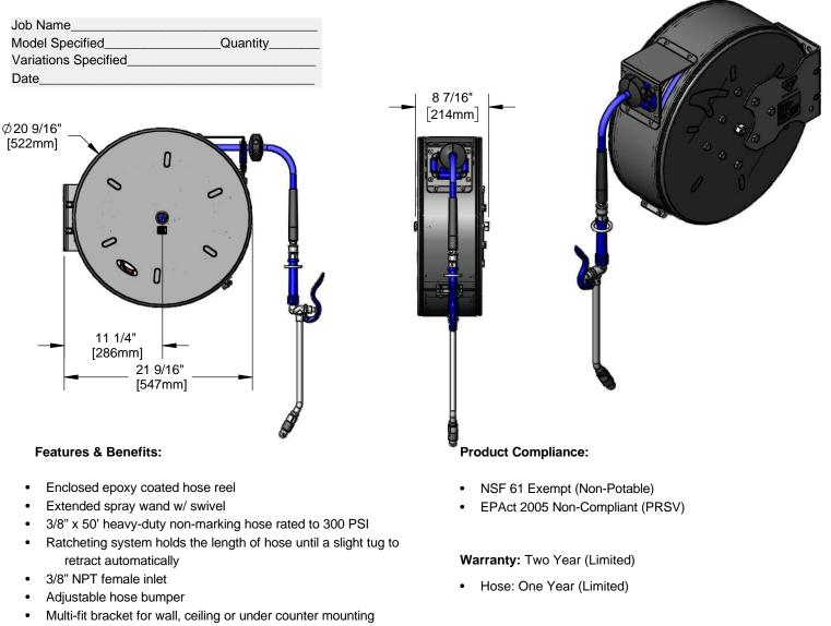
• Material: Epoxy coated steel enclosed reel, wall bracket and chrome plated brass spray valve
