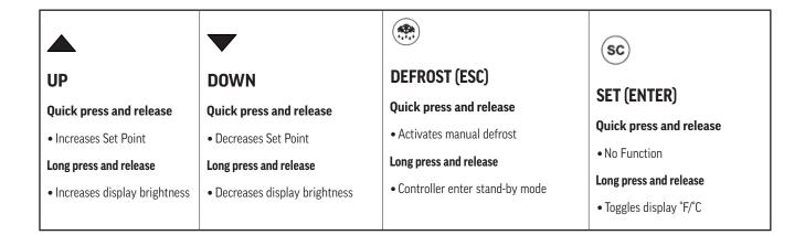
Note: When the controller is in a Standby Mode, a blue dot will be displayed as shown here. To switch out of Standby Mode, push and hold the Defrost button until the display reads ON.
