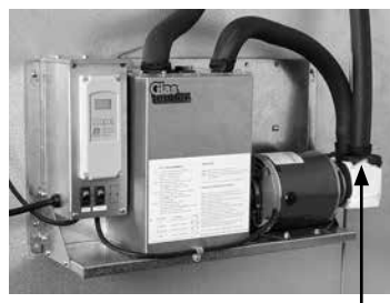
Connect glycol recirculating line from pump outlet 1/2" barb fitting to the beer line set.
