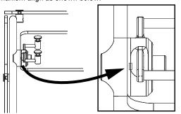
When the notches align, the Adjustable Breath Guard is in the correct NSF 2 position.
