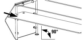
2. Gently lift the glass to reduce the weight resting on the locking hinge and press the release button.
