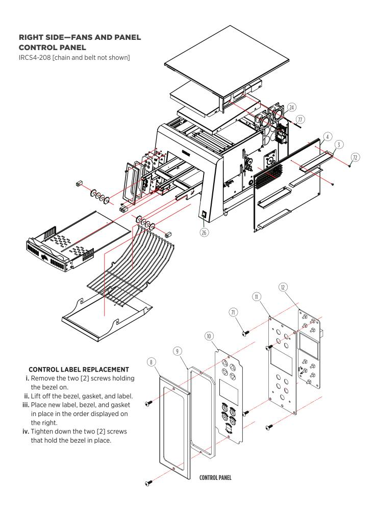
Side references are from the operator's point-of-view—from the front of the unit. Items labeled "NS" are non-serviceable. Items labeled "NP" are not pictured.
