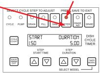
Change STEP START TIME or STEP DURATION using ARROW buttons (adjustments are made in 0.25-second increments).
