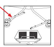
**POWER UP** To place the machine in standby, flip "OFF/ON/FILL" switch to "ON" position.
