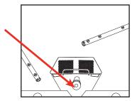
4. Wash tub must be completely filled before operating wash pump to prevent damage to components. Once wash tub is filled, machine is ready for operation.
