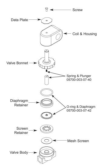
Complete 115 Volt Solenoid Valve Assembly 04810-100-53-00
