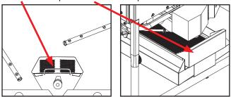
2. Drain stopper is installed.
