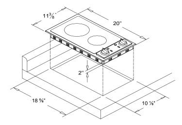
**NOTE:** When making the countertop, radius the corners of the cutout (1/4" radius is typical). This will prevent cracking of the countertop. Follow the countertop manufacturer's instructions regarding the minimum corner radius and reinforcement of corners.
