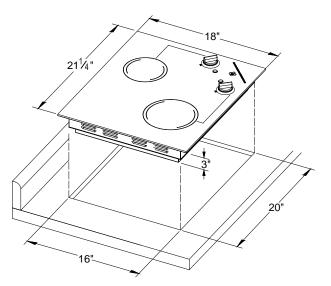
**NOTE:** When making the countertop, radius the corners of the cutout (1/4" radius is typical). This will prevent cracking of the countertop. Follow the countertop manufacturer's instructions regarding the minimum corner radius and reinforcement of corners.
