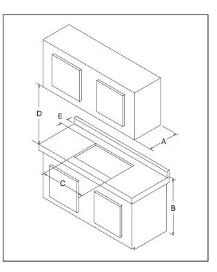
NOTE: Do not install closer than 1/2 inch (12 mm) from any adjacent surface.
