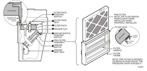
Fig. 6 Filter Installation
