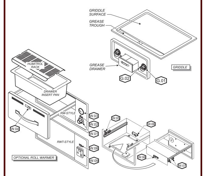
Fig. 3 Griddle & Warmer Drawer Operating Features & Controls
