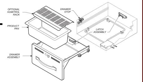
Fig. 7 Roll Warmer Drawer and Pan Installation
