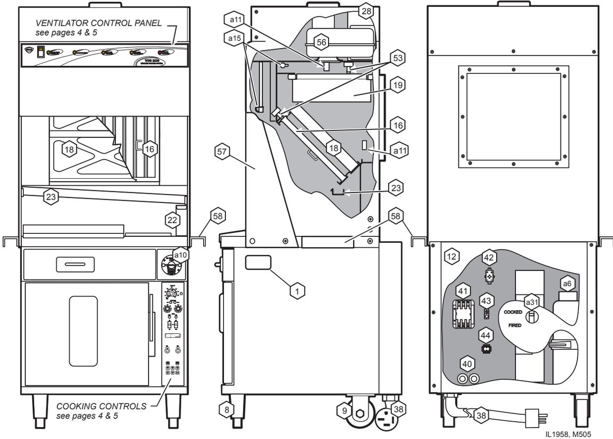
Fig. 1 Ventilator Section Features & Operating Controls
