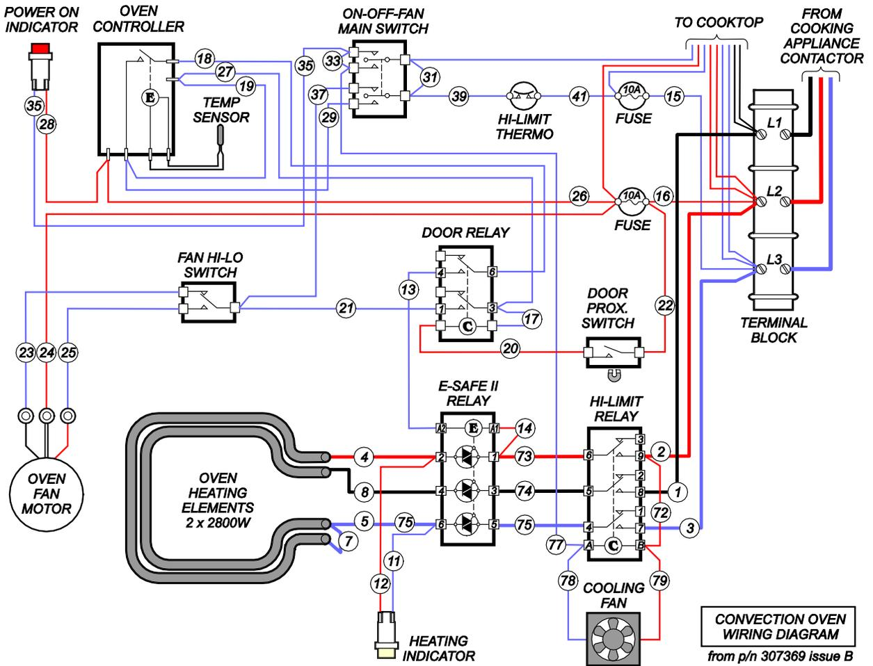
**CONVECTION OVEN WIRING DIAGRAM**
