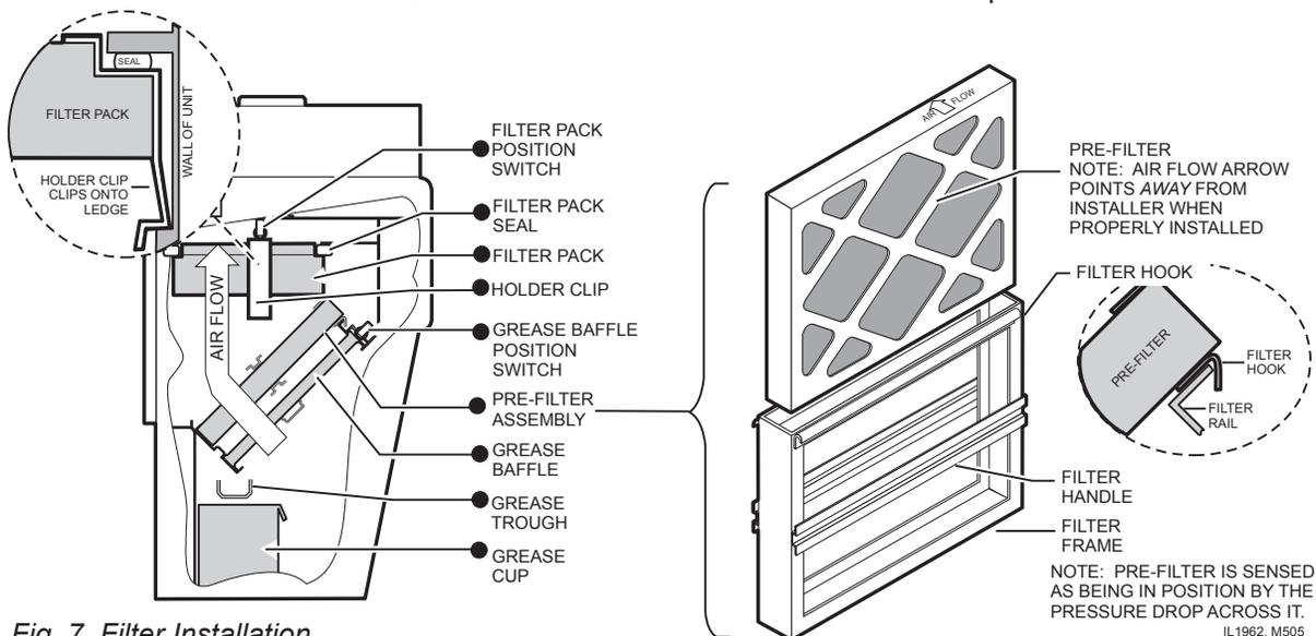
Fig. 7 Filter Installation
