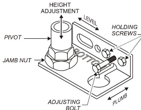
2. Gap between top of door and frame, and between bottom of door and frame must be approximately equal
