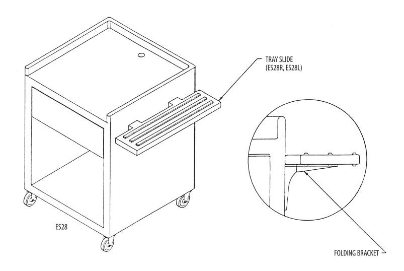
**STEP 1:** To attach Tray Slides, screw 10-32 x <sup>3</sup>/<sub>8</sub> flat head screws though Tray Slide Folding Bracket and into threaded holes in the side of the ES28. Repeat this step with both brackets.
