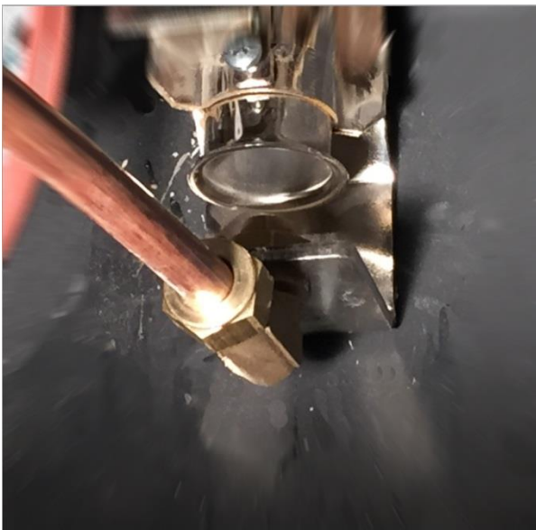
Fig 7.2 Nozzle-holder curve and damper sleeve
