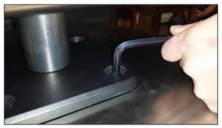
4. Adjust the front height of the upper platen up by turning the adjustment nut counter counter clockwise. Turning the adjustment nut clockwise will lower the front of the platen. Adjust in 180 degree increments, alternating between the two nuts being adjusted.
