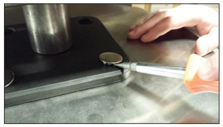
Lower the Top Platen until one side touches to determine which side will be adjusted. In the picture below, the front of the platen could be raised or the back could be lowered.
