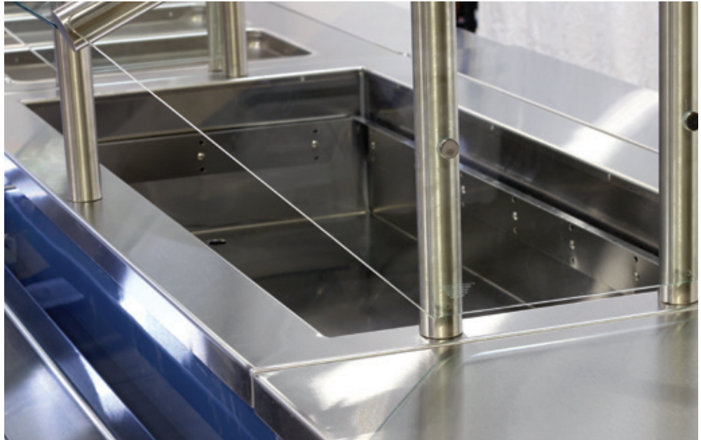
Bloomington Cold Mechanicals (BCM) utilize extra deep wells with recessed, adjustable rails so pans sit beneath the surface of the counter. This allows a blanket of cool air to float above the food, keeping the food fresher, longer.
