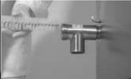
3. Carefully remove the nut and stem assembly. 4. Thoroughly clean the body and tube using the draw-off cleaner brush provided with the Legion Care Kit. 5. When through, rinse with clean water and re-assemble, taking care never to over-tighten the draw-off. It is designed to be hand-tightened only.
