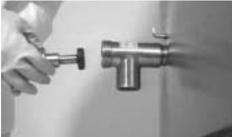
3. Carefully remove the nut and stem assembly. 4. Thoroughly clean the body and tube using the draw-off cleaner brush provided with the Legion Care Kit. 5. When through, rinse with clean water and re-assemble, taking care never to over-tighten the draw-off. It is designed to be hand-tightened only.
