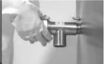
3. Carefully remove the nut and stem assembly. 4. Thoroughly clean the body and tube using the draw-off cleaner brush provided with the Legion Care Kit. 5. When through, rinse with clean water and re-assemble, taking care never to over-tighten the draw-off. It is designed to be hand-tightened only.
