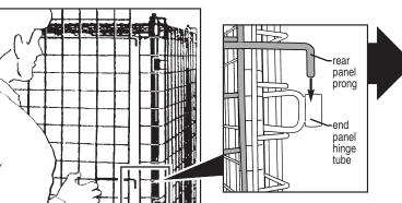
Use the retaining clamps to secure back panel(s) to top shelf (do NOT secure bottom shelf yet).
