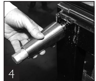
4 Thread leg into cabinet bottom frame rail.
