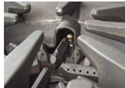
Pilot Lights are protected outside of the spill zone
