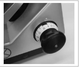
Fig. 71: Slice thickness below "0"
