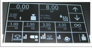
Fig. 54: Automatic operation to target weight
