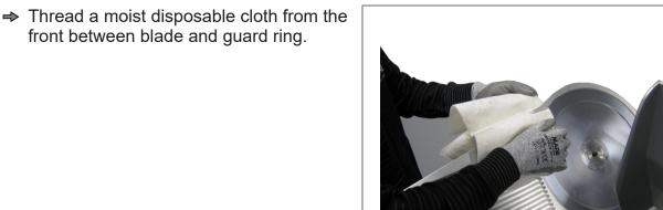
Using your hands, turn blade and disposable cloth; while doing so, slightly press cloth against inner side of the guard ring.
