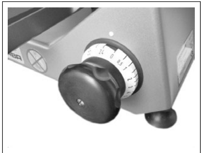
Illustration 33: Slice thickness below "0"
