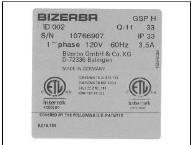
Illustration 7: Rating plate GSP H, example
