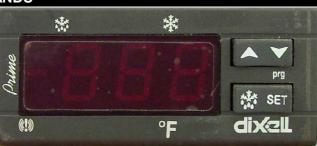
**SET**: To display target set point; in programming mode it selects a parameter or confirms an operation.
