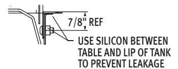
Sectional View Showing Table Connections
