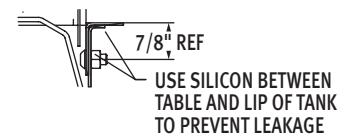
Sectional View Showing Table Connections
