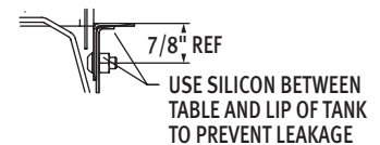
Sectional View Showing Table Connections
