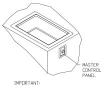
MOUNT APPLIANCE SO THAT THE CONTROL PANEL IS LOCATED TO THE FRONT OF THE FIXTURE.
