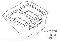
IMPORTANT: MOUNT APPLIANCE SO THAT BOTH THE CONTROL PANEL AND DRAIN MANIFOLD ARE LOCATED TO THE FRONT OF THE FIXTURE.
