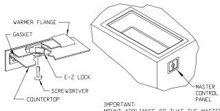
MOUNT APPLIANCE SO THAT THE MASTER CONTROL PANEL ARE LOCATED TO THE
