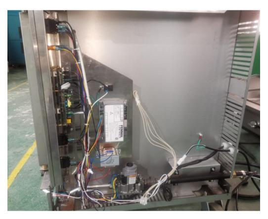
6. Using wrenches to loosen gas line connection to burner manifold.
