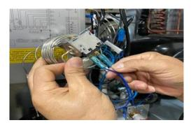
Connect the spade connectors to the bin-stat control.
