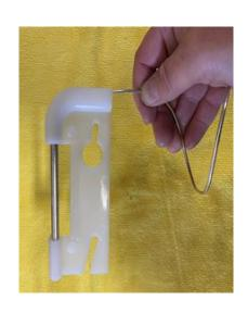
Fit the bulb through the opening & place the bulb tip in the other end.
