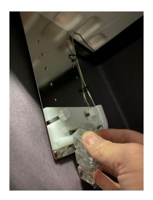
Once install is complete, test the bin-stat's operation by holding ice against the sensing bulb for approixmately 15 seconds.
