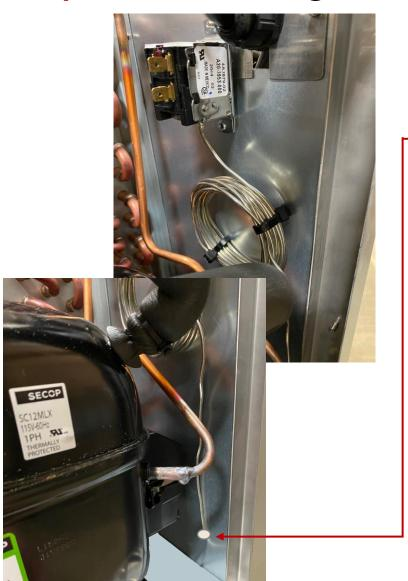
Run the sensing bulb out of the hole made and use the rubber grommet to seal the hole.
