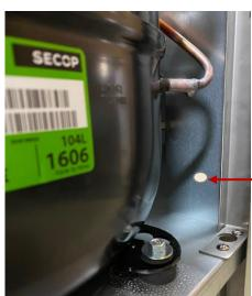
Mount the bin-stat control to the inside, back panel of the ice machine by utilizing the existing screw to the left of the power cord, and then drilling one 3/16" hole below that, through the back panel, and fastening it with the provided screws.
