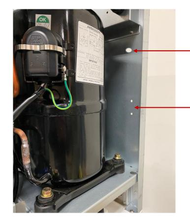
Bulb hole is 5-¾" down from top & 1-¾" from side. First bin-stat hole is 10-¾" down from top & 1-¾" from side. Second bin-stat hole is  $2^{-3}/_{16}$ " down from first hole.
