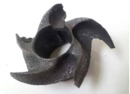
Impeller damaged from high acid solution
