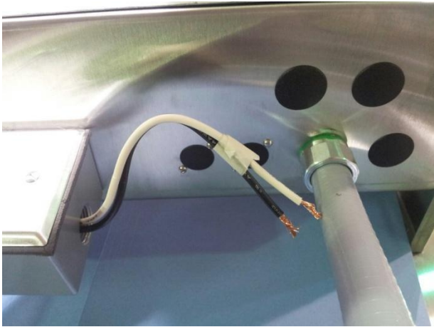
Showing power connection for 120v wiring
