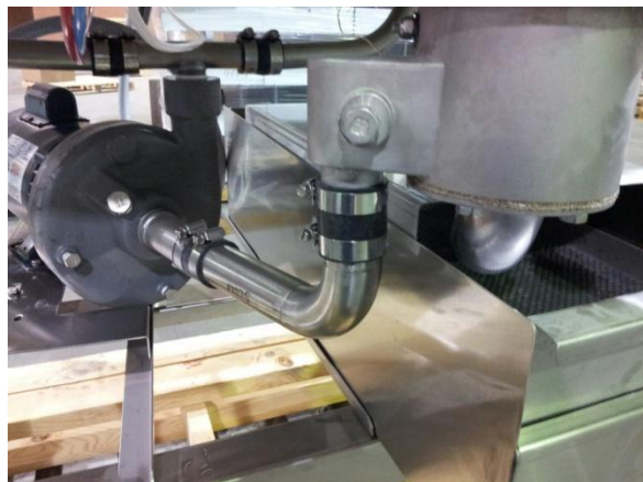
Single Pump, intake and discharge manifolds
