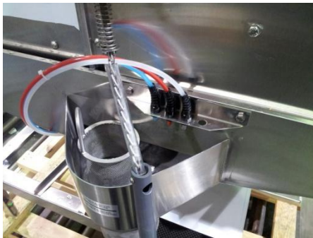
Showing sump, drain ball, water-level decal, chemical tube, SS filter
