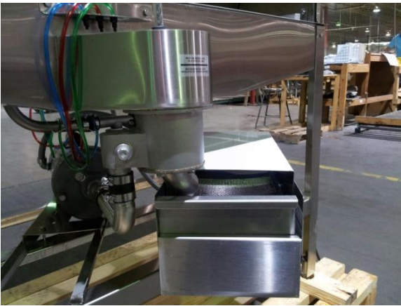
Showing scrap box as installed on 5CD R-F
