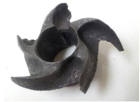
Impeller damaged from high acid solution
