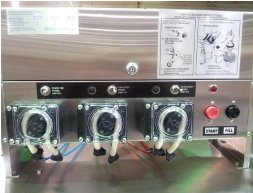
Showing chemical detergent, rinse, sanitizer external pumps
