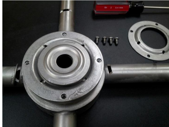
Remove top shell, exposing top bearing race
