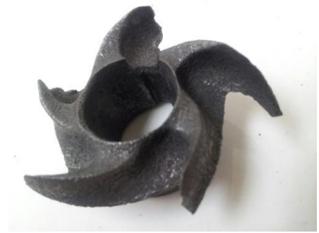
Impeller damaged from high acid solution
