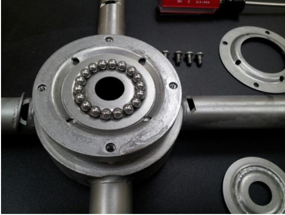
Top race removed, ball bearings for replacement
