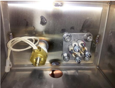
Showing thermostat and sustainer heater terminals*
