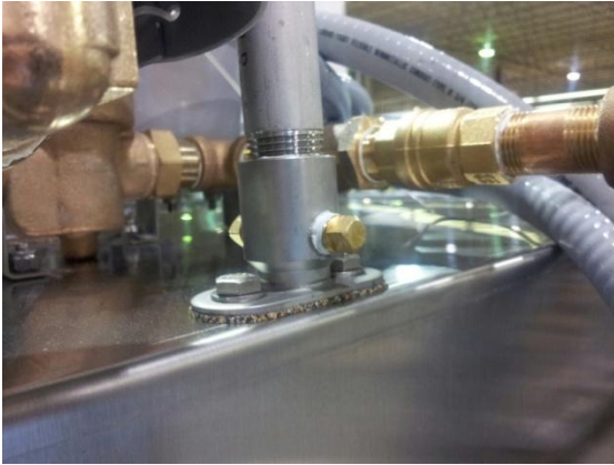
Mixing chamber with two 1/8" pipe threaded port
