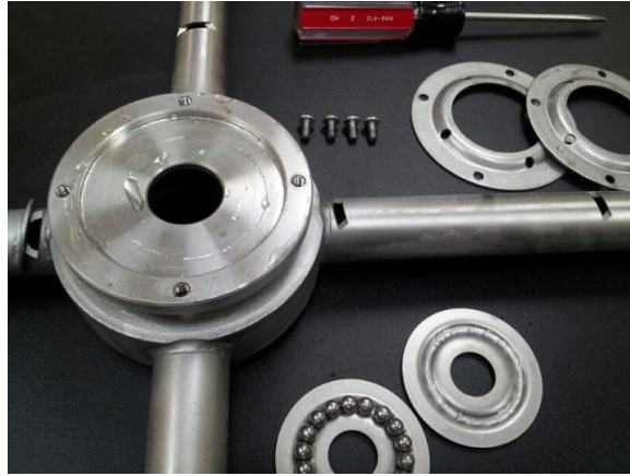
Races are interchangeable, capture shells are also
