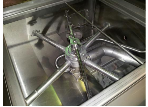
Final rinse arm twisted into transfer tube
