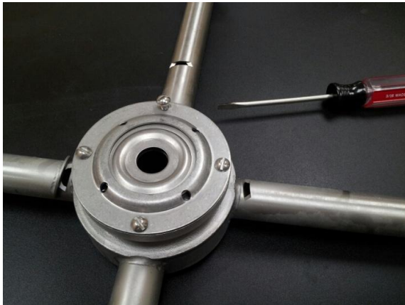
Remove 4 screws and lift top shell
