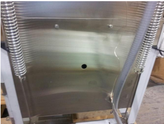
Showing back of tank, 7/8" detergent bulkhead fitting hole
