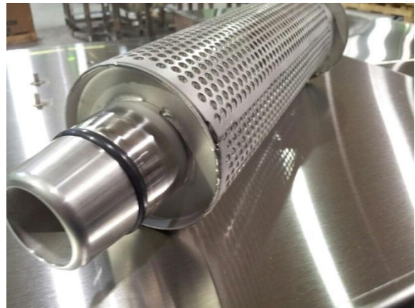
Pump filter and drain plug, note O-ring seal
