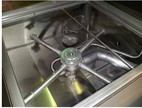
Wash arm w/bearing installed on base
