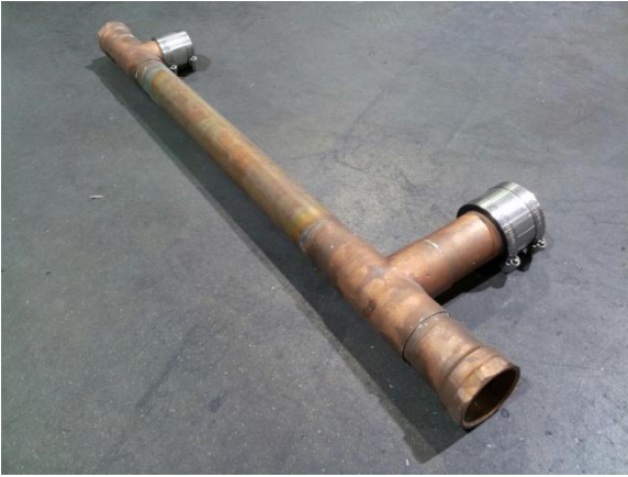
HT-25 drain manifold with “no-hub” connectors
