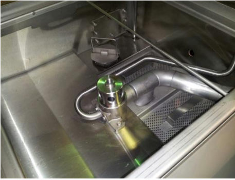
Showing spray arm base &amp; transfer tube
