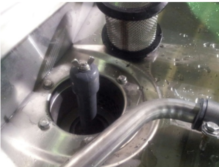
Showing sump, drain ball, pump filter
