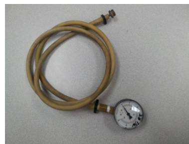
Spray arm pressure tester #088-1048
