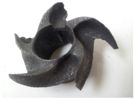
Impeller damaged from high acid solution
