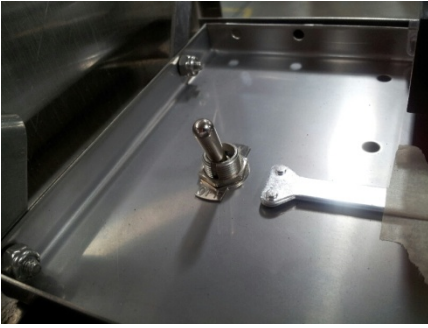
De-lime switch in control box
