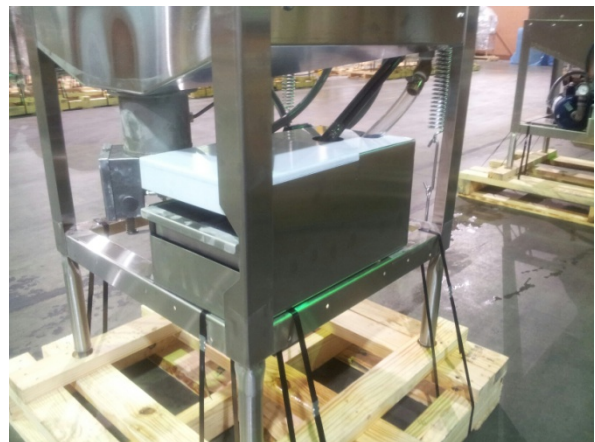
L-3DW-S scrap box in-frame mounting
