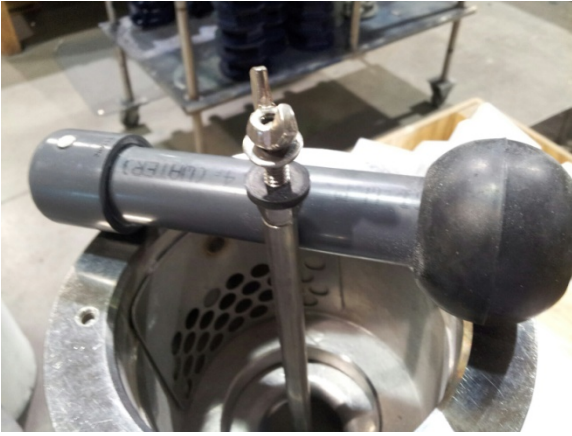
Drain ball assembly, note rubber washer on push rod
