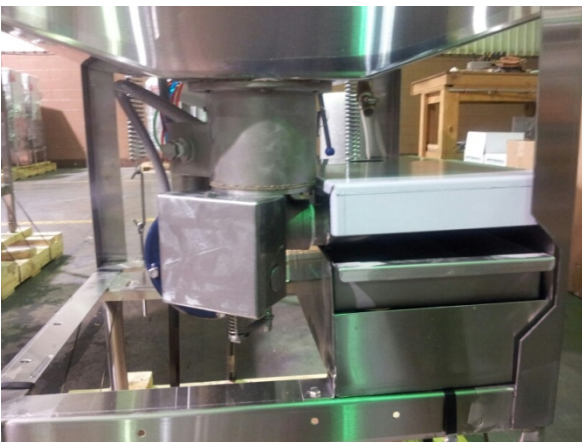
Showing L-3DW-S internal sump and scrap box
