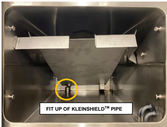
Figure 3-3 KleanShield™ Installation (Model 22CET3.1 Shown)
