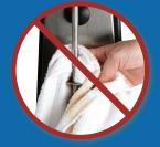
Wiping down spindles with a rag invites cross-contamination
