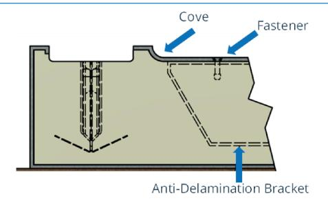
Withstands foot or cart traffic, loads approved up to 1,000 lbs. psf without the need of plywood. Simple floor rating to avoid confusion, rated for foot and cart traffic.
