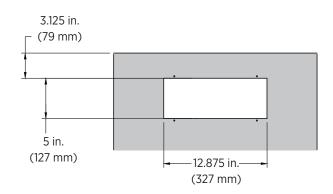
The unit's overall depth is 12.125 inches (308 mm) and will sit approximately 11.75 inches (298 mm) below the counter surface depending on counter thickness.
