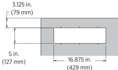
The unit's overall depth is 12.125 inches (308 mm) will sit approximately 11.75 inches (298 mm) below the counter surface depending on counter thickness.
