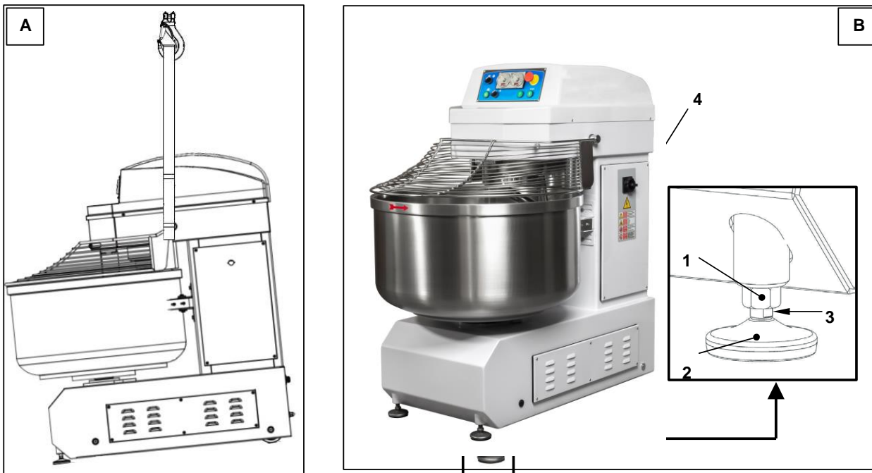
Figure 10 - Lifting the machine with a strap and adjustment of the support feet on the ground
