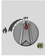
2. Light the pilot adjacent to the main burner. Adjust the pilot valve screw until the pilot flame has a slight yellow tip.
