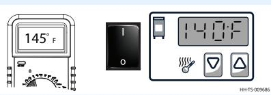
5. If the multimeter temperature and the Actual temperature don't match, **press** and **hold** the Up and down arrow buttons ② for eight (8) seconds. The control will display the previous calibration offset value or 0.
