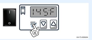
8. Allow the drawer warmer to re-stabilize and **compare** the temperature again. Tolerance at  $140^{\circ}F$  ( $60^{\circ}C$ ) is +/-  $8^{\circ}F$  (+/- $4^{\circ}C$ ). Tolerance at  $180^{\circ}F$  ( $82^{\circ}C$ ) is +/-  $10^{\circ}F$  (+/-  $6^{\circ}C$ ).
