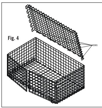
4. Attach the top at a 45° angle, then push in to engage the hooks with the back of the cage.
