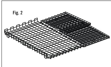
2. Remove all card board and unfold the unit so that the back of the unit lies flat.
