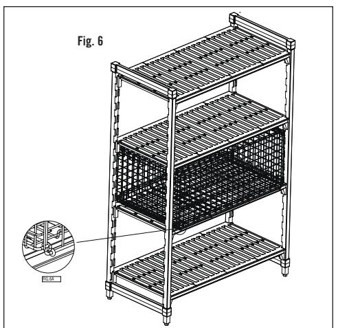
6. Insert the cage into the shelf of the Camshelving® unit. The metal posts hook under the front and back of the traverse. (Fig. 6A)
