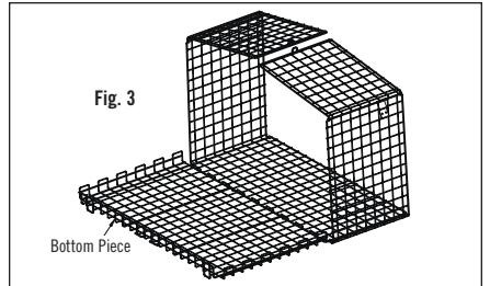
3. Unfold the doors until the unit forms a rectangle. Fold unit down over bottom piece.
