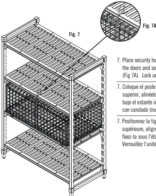
7. Place security hook over top shelf, line up with the doors and secure under bottom shelf (Fig 7A). Lock unit with padlock (not included).
