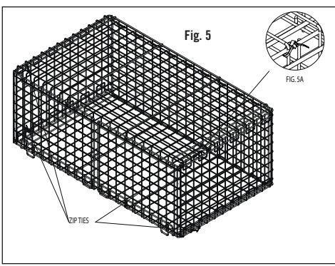
5. Close the top and temporarily secure top, bottom and sides with provided zip ties. (Fig 5A)
