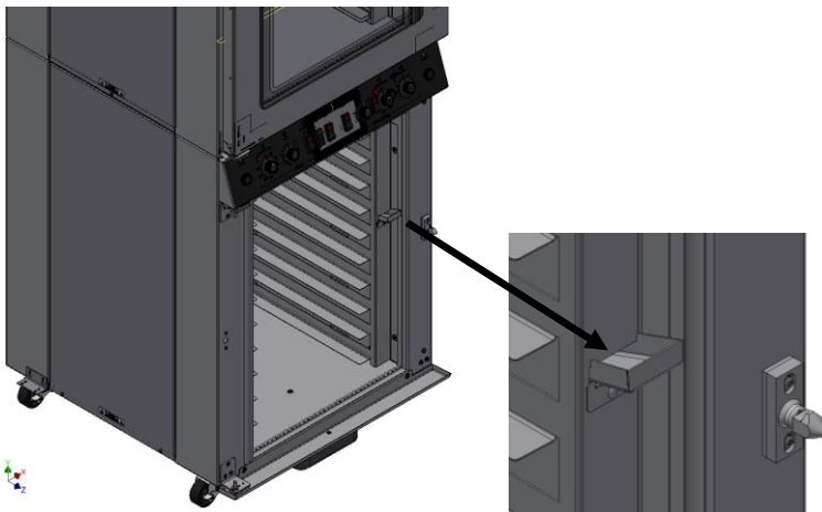
Fig. #2- Manual Fill Water Chute
